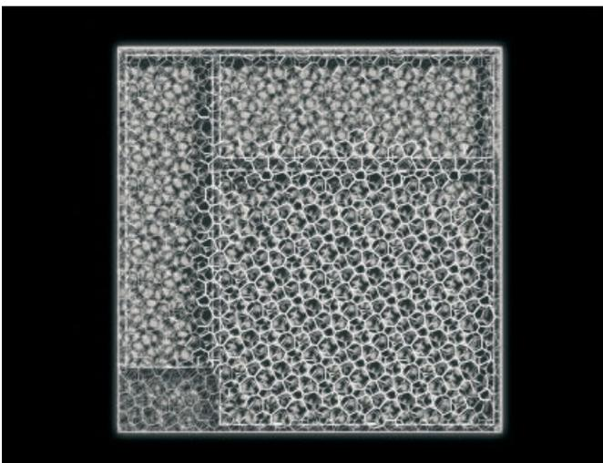
Watercube digital structural model. The mathematics of foam geometries are used to produce the structural array, ensuring a rational optimised and buildable structural geometry.
