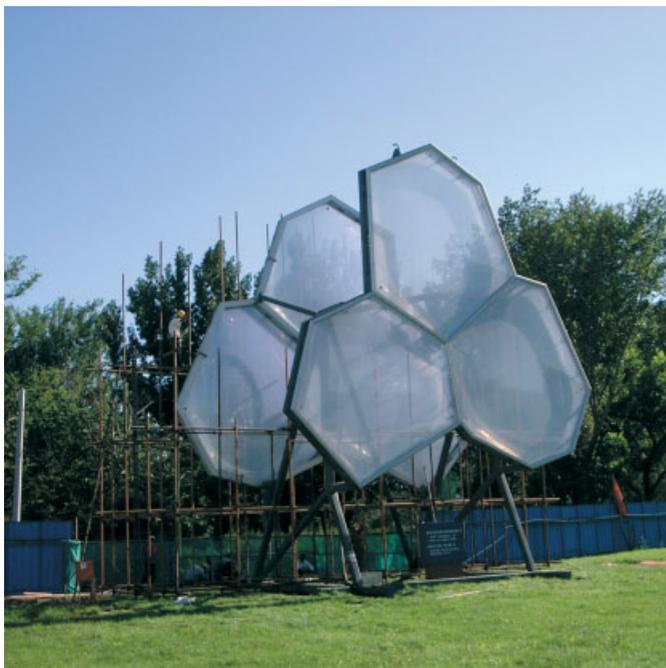
Watercube physical prototype; cells and ETFE cushions fabricated for the testing of environmental and structural behaviour, and confirmation of production logics.
